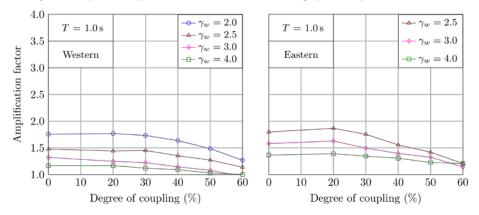
Figure 5. Influence of DOC on seismic shear amplification factor, T = 1.0 s.
