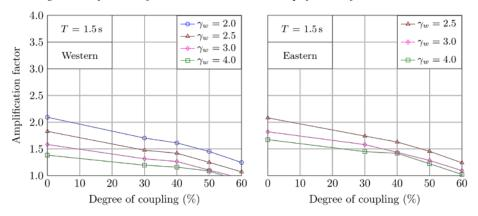
Figure 6. Influence of the DOC on seismic shear amplification factor, T = 1.5 s.
