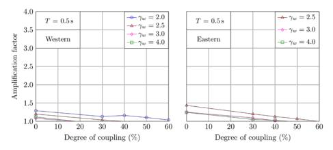
Figure 4. Influence of the DOC on seismic shear amplification factor, T = 0.5 s.
