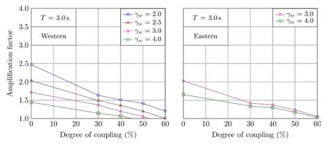
Figure 9. Influence of the DOC on seismic shear amplification factor, T = 3.0 s.
