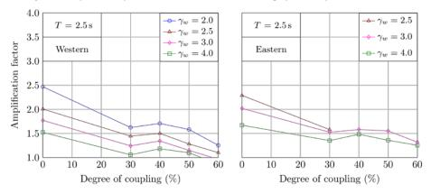
Figure 8. Influence of the DOC on seismic shear amplification factor, T = 2.5 s.
