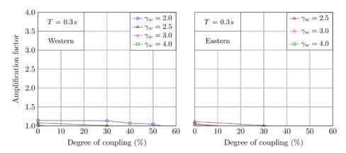
*Figure 3. Influence of the DOC on seismic shear amplification factor,* T = 0.3 *s.*
