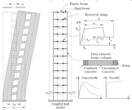
Figure 2. Multilayer beam-column elements on OpenSEES.
