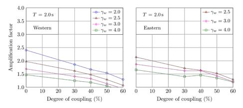
Figure 7. Influence of the DOC on seismic shear amplification factor, T = 2.0 s.
